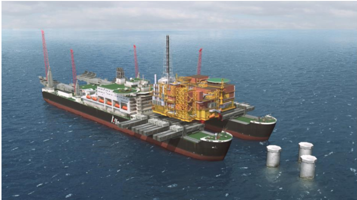
Figure 4.6 The Brent Delta topside secured on the SLV Pioneering Spirit ready for transportation to the nearshore transfer site.
