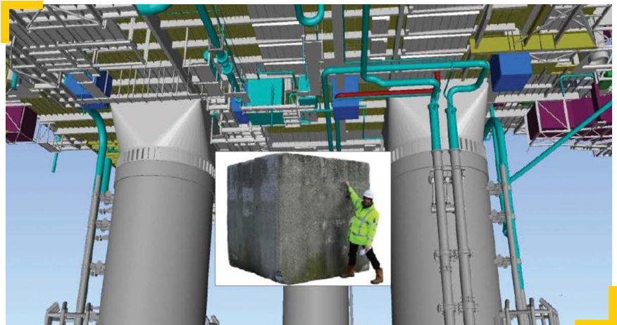
Underside of Brent Bravo – Introduce 6 mass concrete lift points (shown in blue, 4 south and 2 north)
